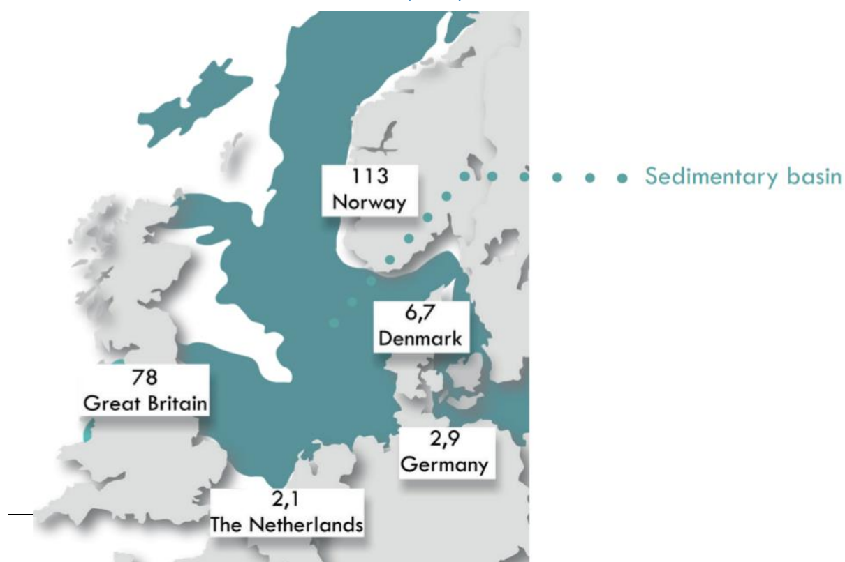
Figure 3-1 CO 2 storage potential around the North Sea, in billion tons (Acatech, CCU und CCS-Bausteine fuer den Klimaschutz in der Industrie, 2018)
