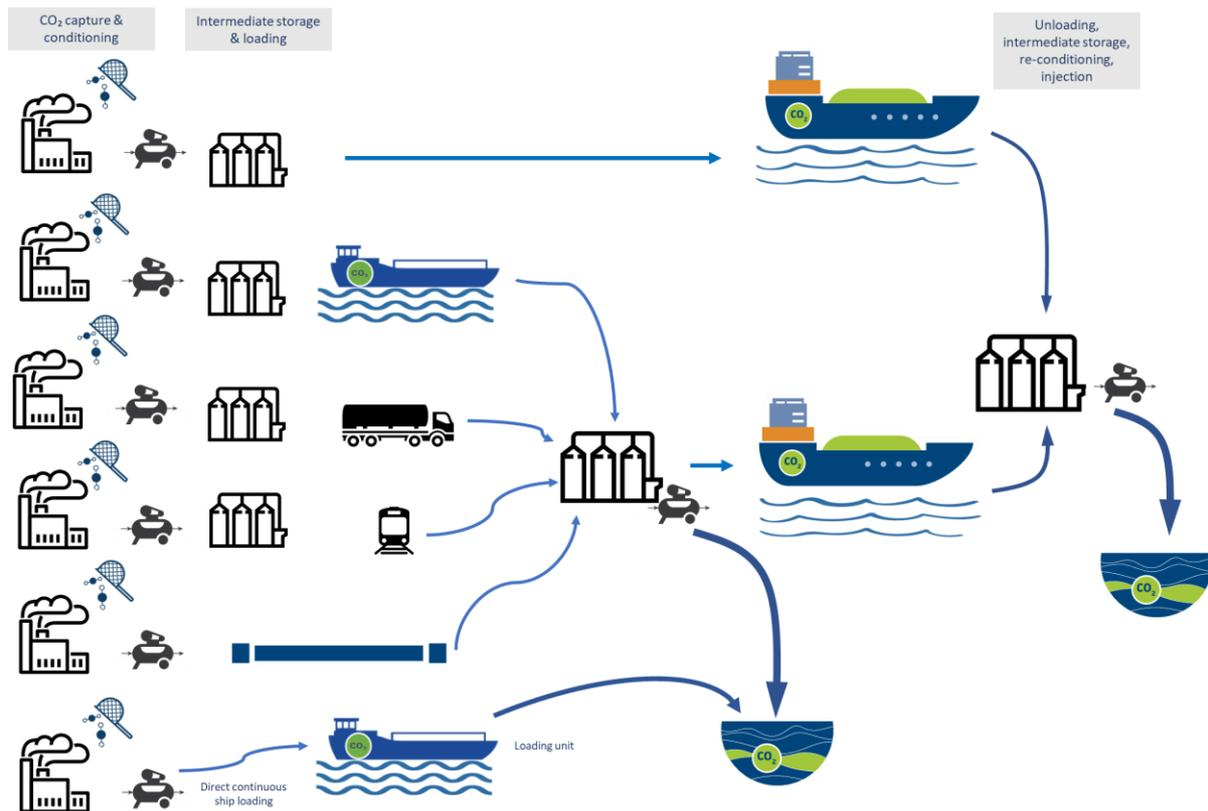
Figure 1 Simplified value chain alternatives for CCS. Note: Pumping not shown. A list of icons is in Table 2.
